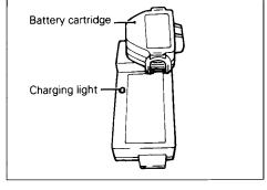
battery charger. Insert the cartridge fully into the port so that it rests on the charger port floor.
